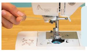
• Bring the thread around the needle threader with the thread seated in number 7 position. Lower the presser foot.
