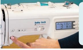
Push the start/stop button to activate the bobbin winder.
