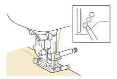
Press the (1) (Thread cutter button) to trim the upper and lower threads.
