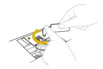
Turn the handwheel to check that the feed dogs move smoothly and do not contact the edges of the slots in the needle plate.
