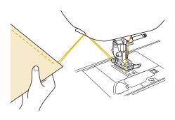
When the needle has stopped moving, raise the presser foot and remove the fabric.
