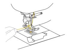
Pull up the bobbin thread, pass it under the presser foot and pull it about 10 cm (4 inches) toward the back of the machine, making it even with the upper thread.
