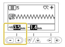
Each press of "-" makes the zigzag stitch narrower.
